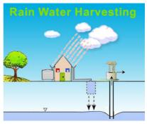
Minimum Net Volume (m<sup>3</sup>) = 0.25 (Minimum percentage of Terraces & Roof) x Area of roofs and Terraces (m<sup>2</sup>) x 0.8m/m<sup>2</sup>/year (Rainfall) x 0.6 (Factor of Evaporation, 1st rain, wastage, etc...)
